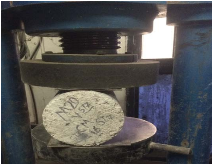
Fig 8 Split Tensile Test
